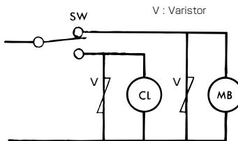
When using the standard power supply box (TMP-type), because a discharge circuit is included, the above procedure is not necessary.
