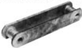
2. Wear from Conveyed Materials
