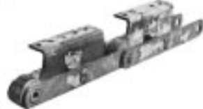
3. Wear from Corrosion
