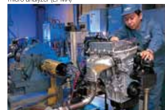
Testing a timing chain drive system
