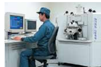
Cutting-edge materials analysis with an electron probe micro analyzer (EPMA)
